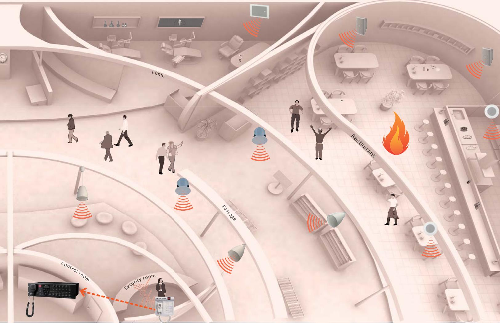
this code are intended to be used to communicate critical emergency communication and/or mass notification, in conjunction with other equipment, within a building or outdoor area. The system is to notify occupants of emergency procedures or events, including; fire, weather emergencies, amber alerts, terrorist activities, and more.
