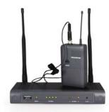
Multi-function receiver, 16 switchable frequencies. Latest PLL quartz tuning technology. Features include LEDs on receiver showing Power On, AF Peak level, RF Level and Diversity Channel A or B. Rear mounted detachable antennas and variable gain jack plug output. Beltpack system supplied with omni-directional condenser mic and instrument cable - both with locking 3.5mm jack. Battery life in excess of 8 hours.
