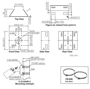
Designed to mount the TOA CCTV Cameras on a pole in conjunction with the optional YS-60B.
