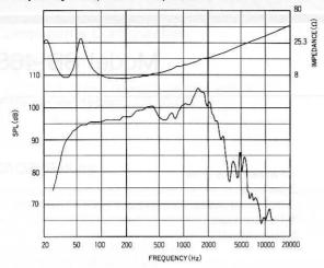
Measured in an anechoic environment at 1 watt and 1
