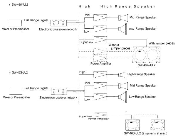
2. System using electronics crossover network and 2 or 3 power amplifiers.
