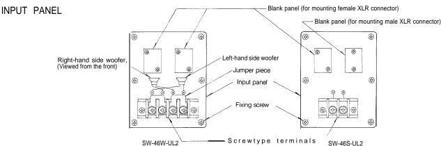
The two woofers of the SW-46W-UL2 are connected in parallel when jumper pieces are used (impedance is 4 ohms). Removal of the jumper pieces disconnects the two woofers from each other, allowing each of them to be driven independently by means of their respective
