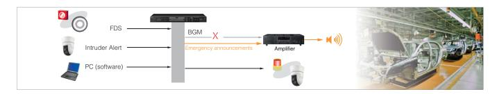
R.E.M. (Recording Endless Message) function enabling operators to create/initiate repeated play back of emergency announcements quickly and evacuate with other occupants before anticipated emergencies such as tsunami
